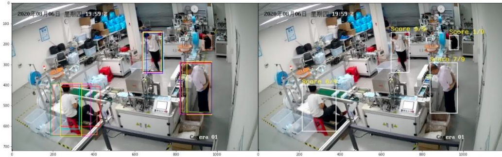
Fig. 2. Left bounding boxes (bbx) of various models, right bbx with a number of models which object recognition agrees – these form an algorithmically created "pseudo ground truth" without any human intervention (video source: 4_APL80).
