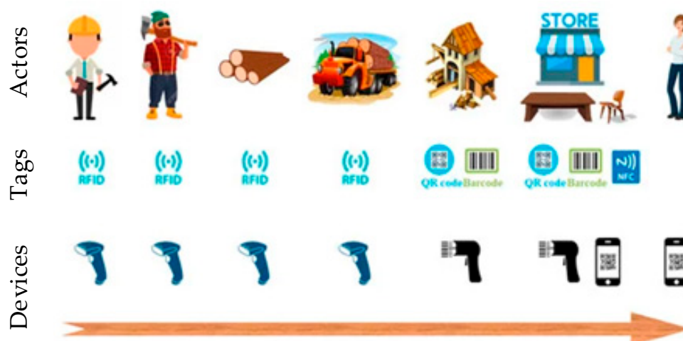
Figure 4. Wood monitoring through RFID, covering the full supply and production chain [90].
